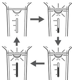
**<When the battery capacity is low>**
